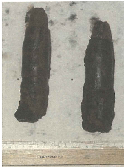
Fig. 4. Recovered 38 mm rounds. Contact corrosion between fuse and shell body is clearly visible.
