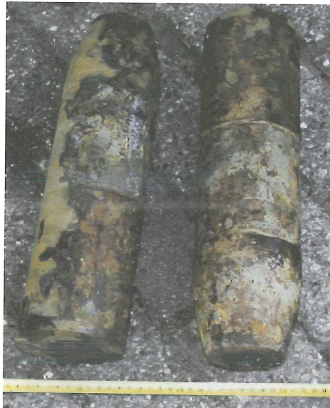
Fig. 6. Recovered 4,2-inch mortar rounds filled with white phosphorus. These rounds were leaking white phosphorus because of contact corrosion between the burster and the steel body.
