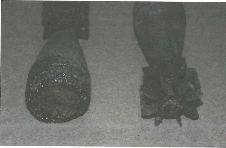
Fig. 5. Recovered 60-mm mortar rounds. Part of the explosive payload is already dissolved in the water. The steel cases are strongly attacked by the sea water; sometimes only a carbon skeleton remains, that could be pulverised easily.
